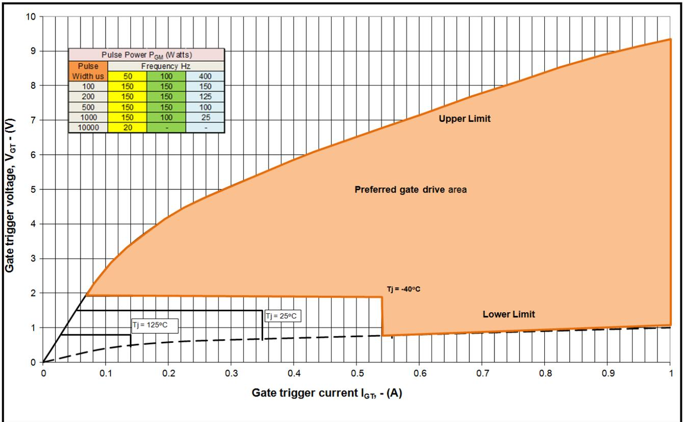
**Fig14 Gate Characteristics**
